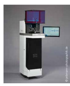
LAwave measuring system for fast and non-destructive characterization of small and medium-sized components.
